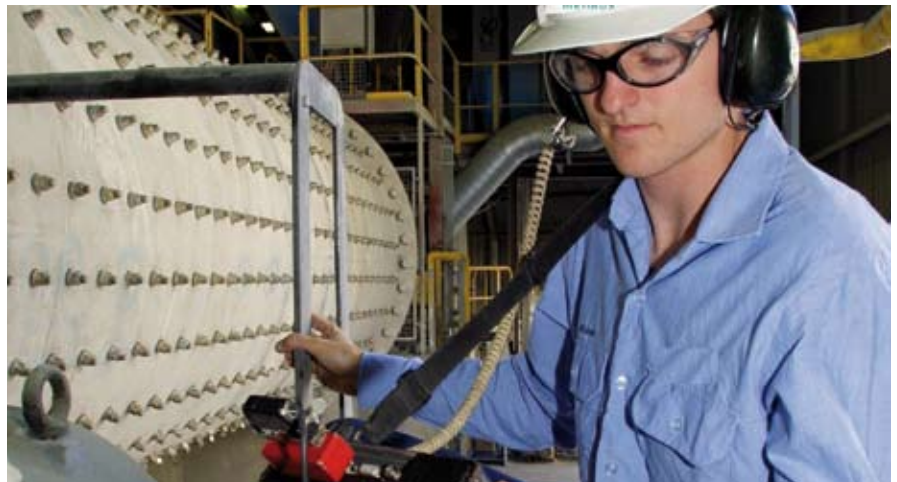
A Metlabs engineer conducting condition monitoring
